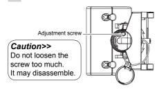
Tilt the bracket about 45° and pass through the wire.
