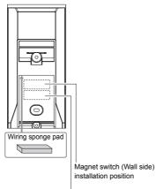
Magnet switch (Base side) installation position
