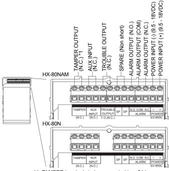
\*1: TAMPER terminals to be connected to a 24 hour supervisory loop.
