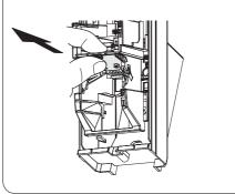
2 Move the flap to the position that corresponds with the desired detection distance.
