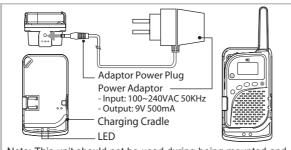
Note: This unit should not be used during being mounted and charged on the charging cradle.
