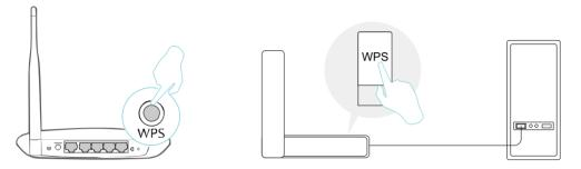
2. Within 2 minutes, press and hold the WPS button on the adapter until WPS Tool opens in the lower right corner of your computer.
