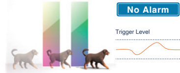
Pets cover only a small area and generate a much smaller signal than humans.
