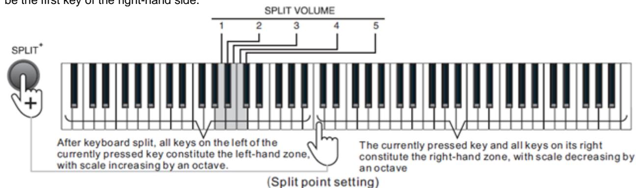
When the piano split function is enabled, the scale of the left-hand zone will increase by an octave, and the scale of the right-hand zone will decrease by an octave. Take the default split point as an example, scales of Keys A0 - G2 # will change to those of Keys A1 - G3#, while scales of Keys A2 - C8 will change to those of Keys A1 - C7.
