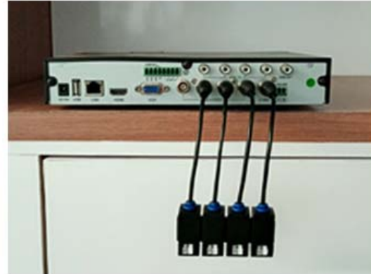
Baluns click together for a neat installation
