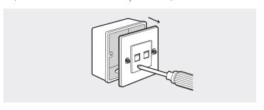
2. Detach the faceplate of the EAP with a screwdriver.
