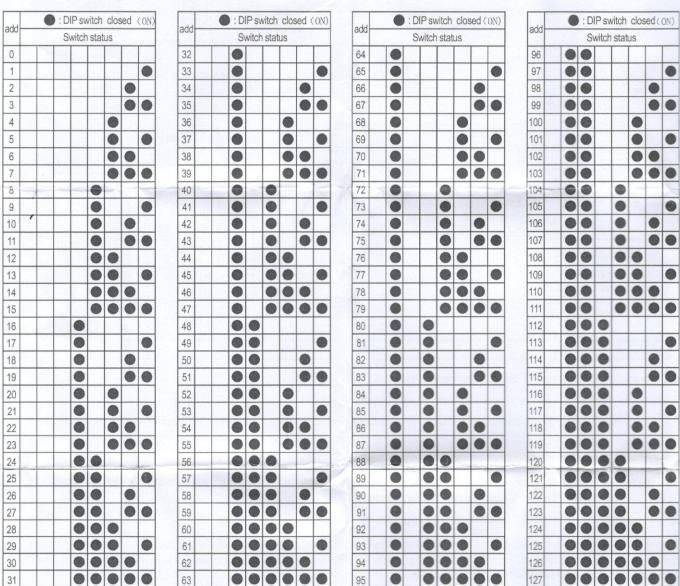
Note: 1. The large-scale bus system alarm panel can connect up to 127 bus equipment through the communication interface. The range of the address DIP switch is 0 to 126.
