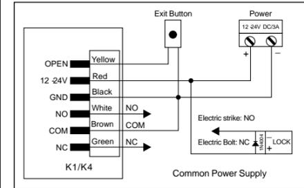
**Attention:** Install a 1N4004 or equivalent diode is needed when use a common power supply, or the keypad might be damaged. (1N4004 is included in the packing)
