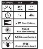
\* The infinitely variable brightness function provides output from 1 lumen to 45 lumens, with corresponding runtime ranging from 1 to 48 hours.
