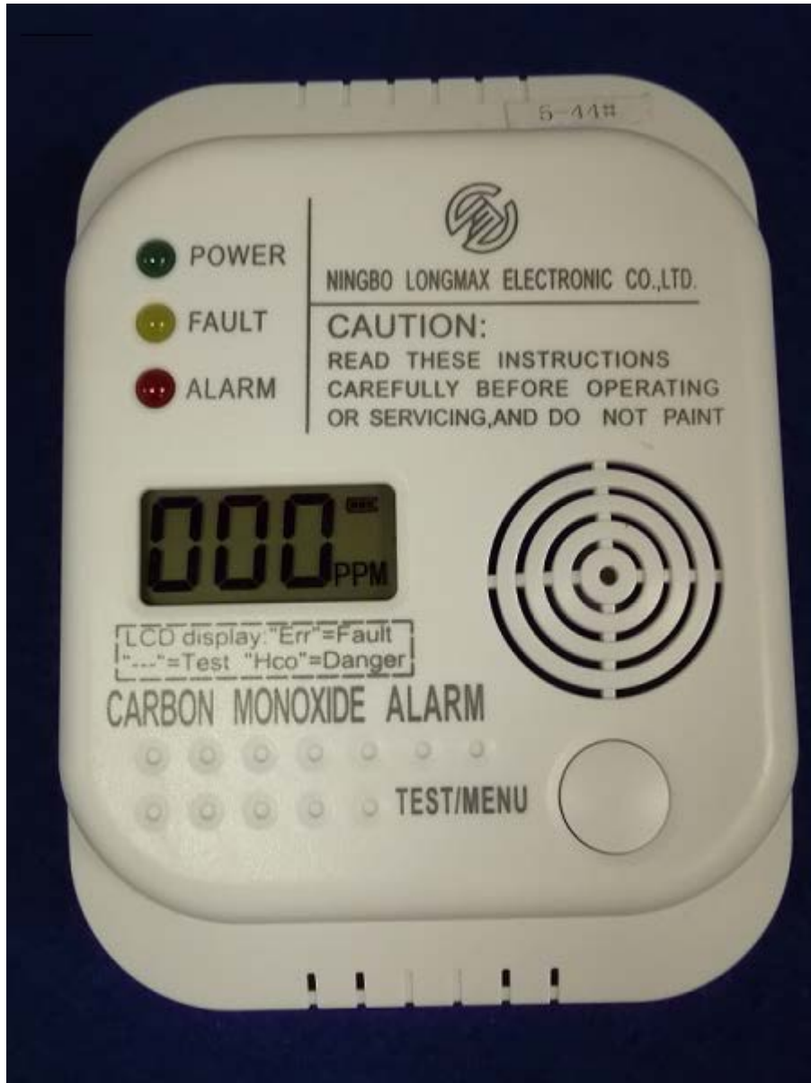
Plate 1: Ningbo Longmax Electronic Co., Ltd LM-201A battery operated (CO) Detector Type B.
