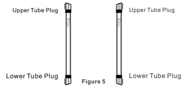
5. Remove upper cover of lower tube plug for TX and RX, it is entering alignment mode after 4 beeps. Adjust it until buzzer doesn't beep. It enters normal working mode after well-alignment.
